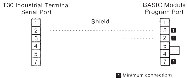
Figure 4.8 T30 Serial Port/BASIC Module Peripheral Port Connections
